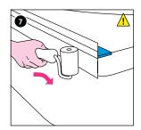
Using the back of your hand or a GABAG application roller, press the FLEXZARGE<sup>®</sup> firmly onto the edge of the tub/tray, paying special attention to the corners.
