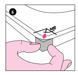
Apply the corner compensation profile to the edge of the tub/tray at an angle of 45°, only where the FLEXZARGE® will be applied later on. Remove the covering film on the outer side.
