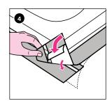
Follow steps 1 to 5 of the installation procedure for all surfaces that require horizontal sealing. Detach the cover strip from the wide grey adhesive.
