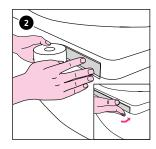
Apply the butyl strip (supplied with the product) in one piece, flush with the upper edge of the tub/tray. Apply it around the radius at the edge of the tub/ tray. Only fit the butyl strip where the GABAG FLEXZARGE® will be applied later on. Place the butyl strip under the tub/tray edge and press everything together firmly. Remove the protective film.
