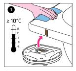
Rub the tub/tray edge thoroughly with a (moist) cleaning cloth, leave to air for 3 minutes and wipe off with a dry cloth: use an adhesive test strip to check whether the adhesive sticks. Do not use on sensitive surfaces.
