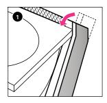
Install the horizontal sealing strip and soundproofing profile.
