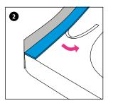
Pull the covering paper off from the underside and press the FLEXZARGE® onto the tub/tray.
