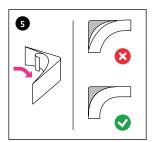
Select the corner compensation profile that matches the tub/ tray edge. The corner profile must be flush with the tub/tray edge. Remove the covering film on the inner side.
