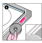
Fit the white soundproofing profile (3×30 mm, perforated) onto the curved tub/tray surround, at the horizontal seal. Perforation at the bottom.
