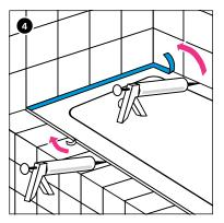
After tiling, pull off the perforated blue tub/tray edge guard profile and prepare the joint with silicone (e.g. Ottoseal® S100 or equivalent) to an adequate width. The remaining piece is used as joint backfill (round cord seal) and to absorb sound.
