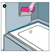
Apply the second layer of composite seal on top of the affixed sealing strip.
