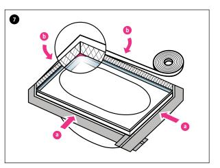
Fit the white soundproofing profile (1×15 mm) b on the rear side of the FLEXZARGE°.
