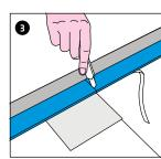
Using the cutter, make an incision into the blue soundproofing profile at the edge of the tub/tray. Place a piece of cardboard underneath for protection.
