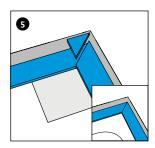
Mitre-cut the blue soundproofing profile, remove any remaining pieces and the tub/tray edge guard, and continue to install the soundproofing profile.
