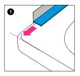
Hold GABAG FLEXZARGE® at a 90° angle to the tub/tray edge. The FLEXZARGE® must be flush with the tub/tray edge.
