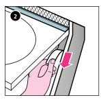
Pull the adhesive strip cover tape away from the narrow grey adhesive and fit flush with the upper edge of the GABAG FLEXZARGE®. Pull off the same area of FLEX-ZARGE® cover tape.
