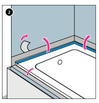
Pull off the cover paper on the rear of the sealing strip and bond it to the dried composite seal. Apply the sealing strip to the seal so that it is flat, with no air trapped inside.
