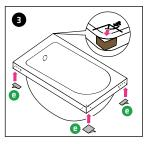
Depending on the installation situation, apply the corner connection pieces (2) below the tub/tray edge and press them on firmly.
