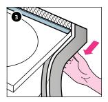
Fit the narrow grey adhesive flush under the tub/tray edge and press it on firmly.
