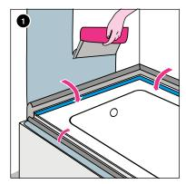
Fold the sealing strip down towards the tub/tray and apply the composite seal to the wall.
