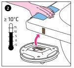
Rub the tub/tray edge thoroughly with a (moist) cleaning cloth, leave to air for 3 minutes and wipe off with a dry cloth: use an adhesive test strip to check whether the adhesive sticks. Do not use on sensitive surfaces.
