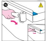
Using the back of your hand or a GABAG application roller, press the FLEXZARGE® firmly onto the edge of the tub/tray, paying special attention to the corners. Affix any projecting butyl strip under the edge of the tub/tray.
