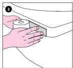
Apply the butyl strip (supplied with the product) in one piece, flush with the upper edge of the tub/ tray. Apply it around the radius at the edge of the tub/tray. Only fit the butyl strip where GABAG FLEX-ZARGE® will be applied later on.
