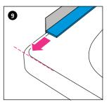
Hold GABAG FLEXZARGE® at a 90° angle to the tub/tray edge. FLEXZARGE® must be flush with the tub/tray edge.
