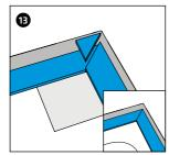
Mitre-cut the blue soundproofing profile, remove any remaining pieces and the tub/tray edge guard, and continue to install the soundproofing profile.
