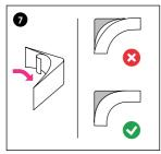
Select the corner compensation profile that matches the tub/ tray edge. The corner profile must be flush with the tub/tray edge. Remove the covering film on the inner side.
