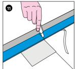
Using the cutter, make an incision into the blue soundproofing profile at the edge of the tub/tray. Place a piece of cardboard underneath for protection.
