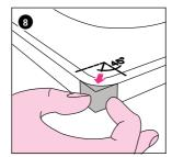
Apply the corner compensation profile to the edge of the tub/tray at an angle of 45°, only where the FLEXZARGE® will be applied later on. Remove the covering film on the outer side.
